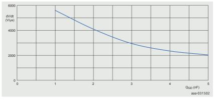
Figure 23 | External  $C_{GD}$  effect on the synchronous rectifier MOSFET
