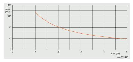
Figure 21 | External  $C_{GD}$  effect on controlling MOSFET turn-off
