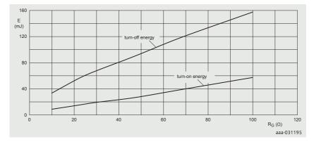
Figure 17 | Effect of varying R<sub>G</sub> on switching loss (example values only)
