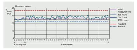
Figure 1 | Dynamic R<sub>DS(on)</sub> measurement during HTRB
