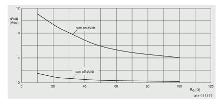
Figure 19 | Effect of varying R<sub>G</sub> on turn-on dV/dt and turn-off dV/dt (example values only)
