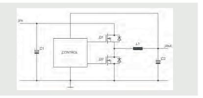
Figure 14 | Synchronous DC-to-DC down-converter
