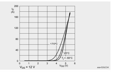
Figure 15 | Transfer characteristics; drain current as a function of gate-source voltage; typical values
