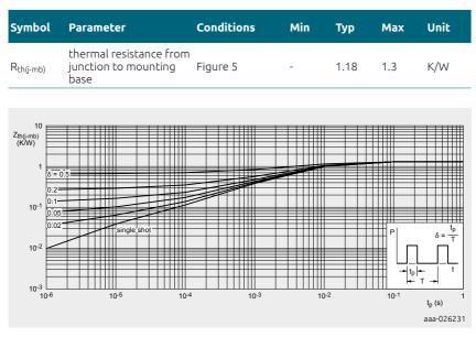
**Figure 5** | Transient thermal impedance from junction to mounting base as a function of pulse duration.
