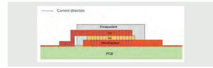
Figure 6 | LFPAK package MOSFET current path
