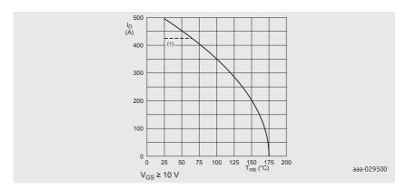
(1) 425 A continuous current has been successfully demonstrated during application tests. Practically the current will be limited by PCB, thermal design and operating temperature.
