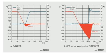
Figure 3 | Reverse recovery charge test result for a GaN FET (left) and a CFD series superjunction Si
