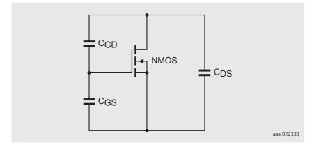
Figure 7 | MOSFET internal capacitances
