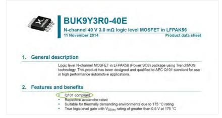
**Figure 5** | Front page of a typical Nexperia automotive data sheet, showing the MOSFET is automotive by highlighting that it is Q101 compliant
