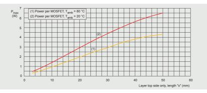
Figure 32 | Maximum permissible power dissipation as a function of copper side length x for LFPAK33
