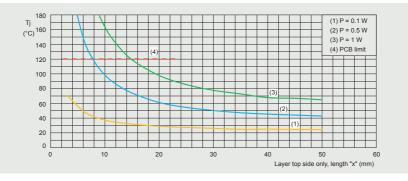
Figure 21 | Junction temperature as a function of copper side length x for LFPAK33
