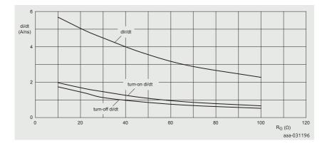
Figure 18 | Effect of varying  $R_G$  on di/dt, dIr/dt and turn-off di/dt (example values only)
