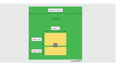
Figure 55 | Split copper area configuration: LFPAK88, single top layer with copper
