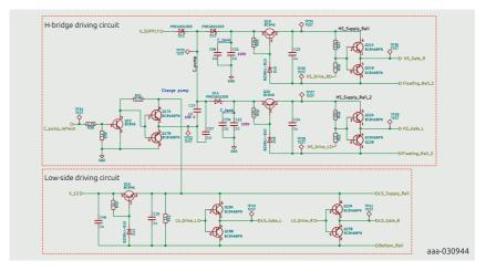
Figure 34 | Driver circuit schematic
