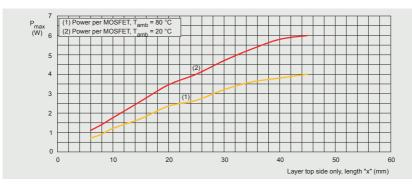
Figure 28 | Power dissipation as a function of copper side length x for LFPAK56D; one MOSFET
