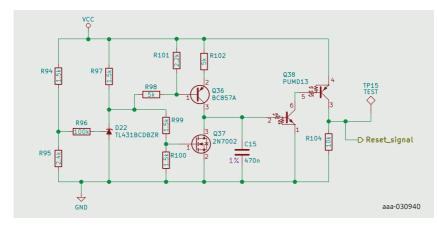
The reset function to activate other function when the  $V_{CC}$  (5 V) supply is stable.
