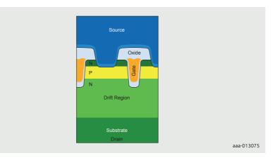
Figure 12 | Trench generation 6 structure
