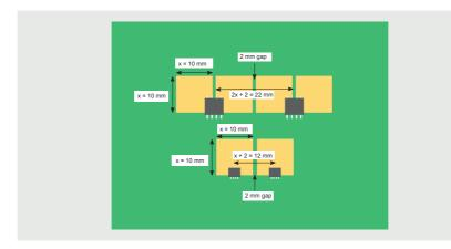
Figure 36 | Copper area configuration: 2 x LFPAK33, 2 x LFPAK56D; separation between MOSFETs
