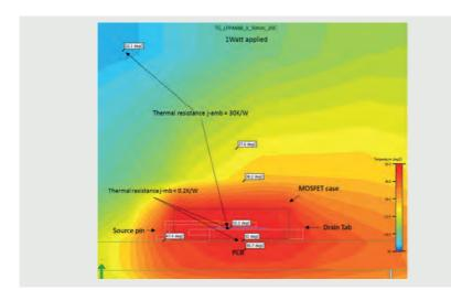
Figure 58 | Thermal resistance LFPAK88: single layer copper profile (50 x 50 mm)
