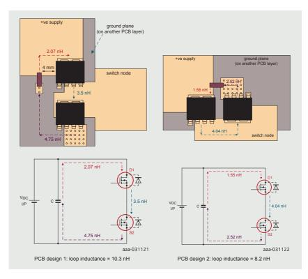
Figure 11 | Half-bridge layout possibilities showing inductances
