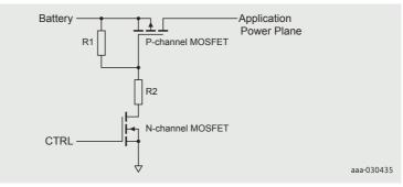
Figure 6 | Load-switch using MOSFETs
