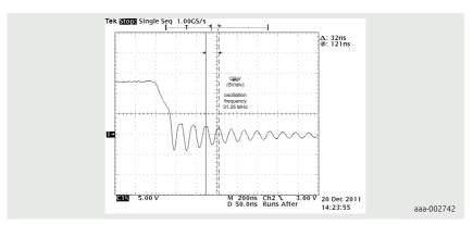
Figure 2 | Reverse recovery-induced oscillation in Q2 V<sub>DS</sub>
