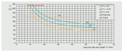
Figure 45 | Junction temperature as a function of copper side length x for LFPAK56
