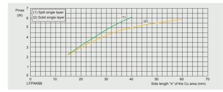
Figure 56 | Maximum permissible power dissipation as a function of copper side length "x" for LFPAK88
