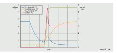
Figure 16 | Waveforms showing the full detail of the gate bounce phenomenon
