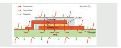
Figure 3 | LFPAK MOSFET - heat transfer model
