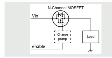
Figure 3 | N-channel MOSFET load switch with high voltage control line
