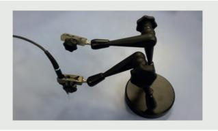
Figure 6 | Probe positioner
