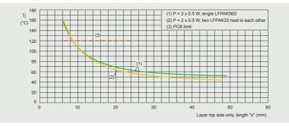
Figure 41 | Junction temperature as a function of copper side length x for 1 LFPAK56D and 2 LFPAK33
