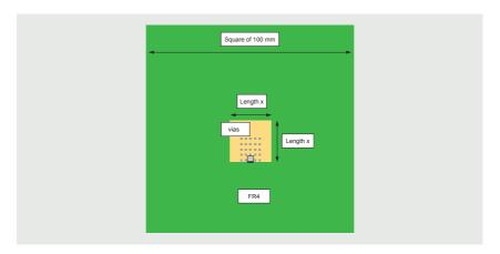
Figure 23 | Copper area configuration: LFPAK56D, 4 layers with vias
