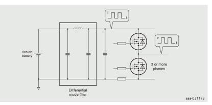
Figure 24 | Sources of electromagnetic noise in a half-bridge circuit
