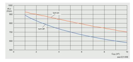
Figure 20  $\mid$  C\_{GS} effect on MOSFET dI/\_pt
