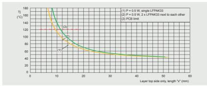
Figure 37 | Junction temperature as a function of copper side length x for 2 LFPAK33
