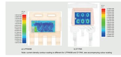
Figure 1 | Current crowding contours for a) LFPAK88 and b) D<sup>2</sup>PAK packages
