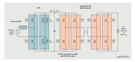
Figure 6 | AC-to-DC PFC stage and isolated DC-DC configuration
