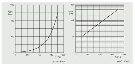
**Figure 22** | I<sub>DSS</sub> as a function of temperature, linear axes
