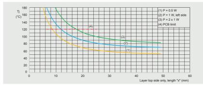
**Figure 17** | Junction temperature as a function of copper side length x for LFPAK56D; one MOSFET conducting
