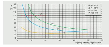
Figure 31 | Junction temperature as a function of copper side length x for LFPAK33
