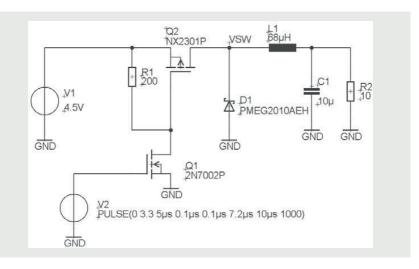
**Figure 7** | SPICE simulation diagram for a simple DC-to-DC down-converter using NX2301P as high-side switch and PMEG2010AEH as low-side Schottky diode.
