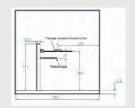
Dimensions in mm. Wiring not shown, but will be placed to avoid interfering with the convection air flow.
