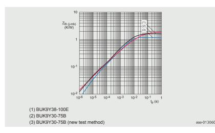
Figure 1 | Comparison of transient thermal impedance
