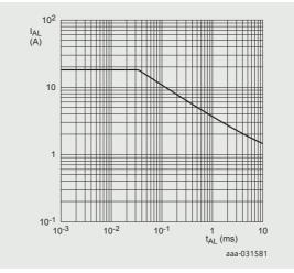
Figure 7 | BUK9K51-60R avalanche rating; avalanche current as a function of avalanche time
