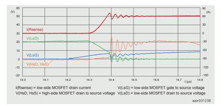
Figure 26 | Measurement turn-on waveform
