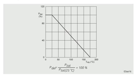
Figure 8 | Normalised total power dissipation as a function of mounting base temperature
