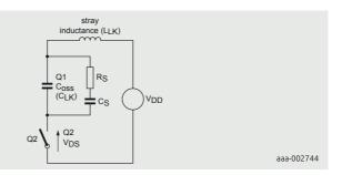
Figure 4 | Equivalent circuit with snubber components R<sub>s</sub> and C<sub>s</sub>
