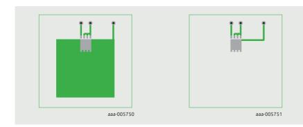
Figure 4 | PCB layout for thermal resistance junction to ambient 1" square pad; FR4 Board; 2oz copper Figure 5 | PCB layout for thermal resistance junction to ambient minimum footprint; FR4 Board; 20z copper
