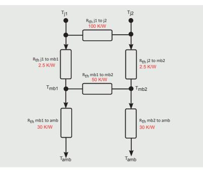
Figure 19 | Thermal resistance configuration
