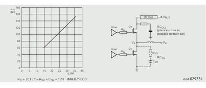
Figure 22 | Snubber capacitance as function of load current
