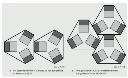
Figure 5 | Layouts using sub groups of three MOSFETs
