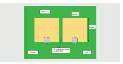
Figure 35 | Copper area configuration: LFPAK33, single top copper layer
