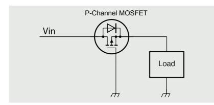
Figure 9 | Reverse current and reverse polarity protection with a P-Ch MOSFET
