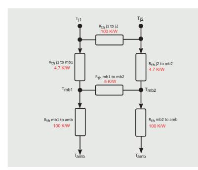
Figure 34 | Dual MOSFET thermal configuration
