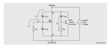
Figure 10 | Power MOSFET showing two possible mechanisms for dV/dt induced turn-on
