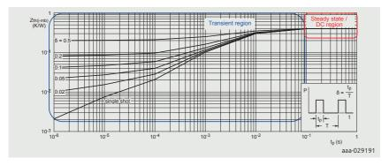
Figure 4 | Transient thermal impedance from junction to mounting base as a function of pulse duration
