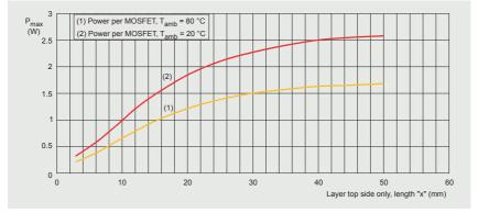
Figure 16 | Maximum permissible power dissipation as a function of copper side length x for LFPAK56D
