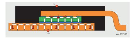
Figure 10 | Thermal path junction to mounting base
