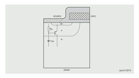
Figure 11 | Physical origin of the parasitic BJT components that may cause dV/dt induced turn-on
