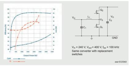
**Figure 8** | Half-bridge boost converter (GaN switch vs Si CoolMOS)
