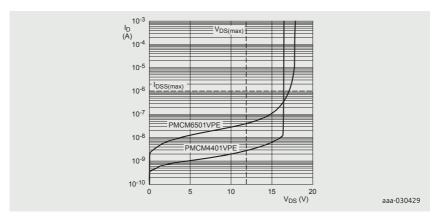
Figure 2 | Drain-source  $I_D$  leakage current as a function of drain-source voltage for PMCM4401VPE and PMCM6501VPE at  $T_j$  = 25  $^\circ\text{C}$
