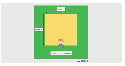
**Figure 49** | Copper area configuration: LFPAK56, 4 layers with vias, the configuration is similar for LFPAK88
