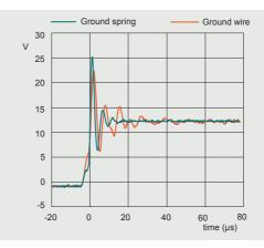
Figure 1 | Switching waveform; probe grounding method comparison
