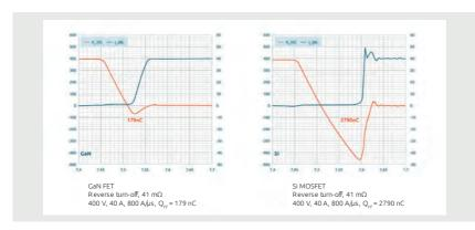
Figure 3 | Qrr, reverse recovery charges for GaN FET vs Si MOSFET
