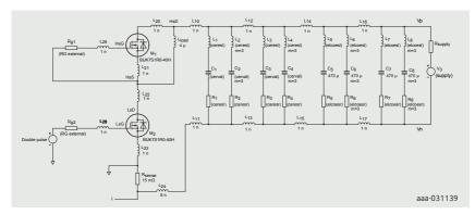
Figure 3 | SPICE simulation circuit for double pulse test circuit
