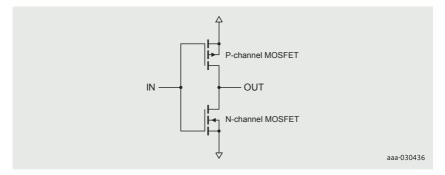
Figure 7 | Inverter using MOSFETs (simplified)
