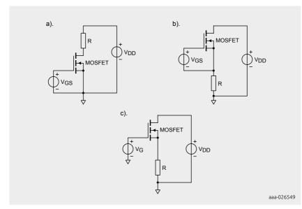
Figure 7 | a) Low side MOSFET b) High side MOSFET driven Gate to Source c) High side MOSFET driven gate to ground
