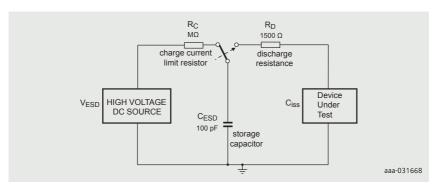
Figure 21 | Test circuit for ESD testing (human body model)
