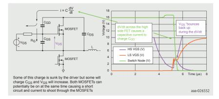
Figure 16 | Dynamic behaviour of a MOSFET half-bridge
