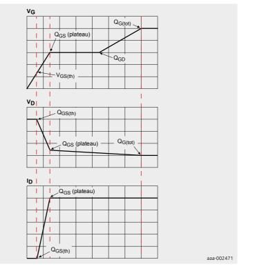
An example of a gate charge curve is shown in Figure 10:
