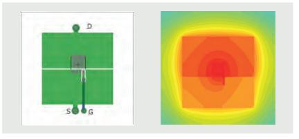
Figure 9 | Test PCB layout 2 and surface temperature profile
