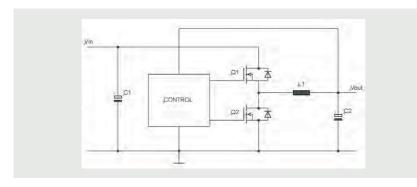
Figure 10 | Synchronous DC-to-DC down-converter (FETs including body-diodes)
