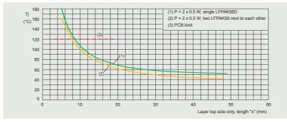
Figure 39 | Junction temperature as a function of copper side length x for 2 LFPAK56 and 1 LFPAK56D
