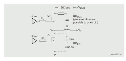
Figure 4 | Half-bridge switching circuit
