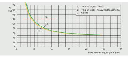
Figure 34 | Junction temperature as a function of copper side length x for 2 LFPAK56D
