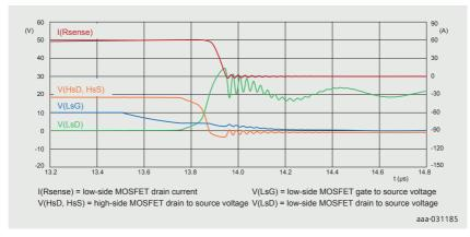
Figure 4 | Turn-off waveform
