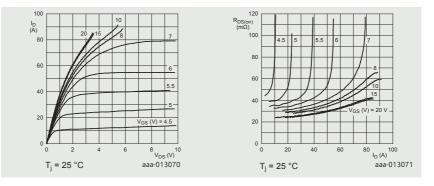
**Figure 25** | Drain current as a function of drain-source voltage: typical values
