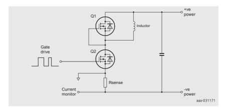
Figure 1 | Simplified schematic diagram of the double pulse test circuit
