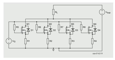
Figure 8 | Schematic diagram of a group of four paralleled MOSFETs intended to operate in linear mode
