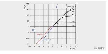
Figure 5 | Cascode GaN HEMFET forward and reverse output characteristics
