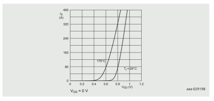
MOSFET data sheets include a  $V_{SD}$  characteristic graph, see Figure 7 below.
