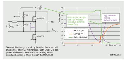
Figure 10 | Dynamic behaviour of a MOSFET half bridge
