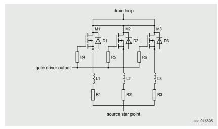
Figure 6 | Schematic diagram showing the stray source inductances and source resistances
