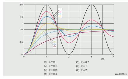
**Figure 5** | Step response of an RLC circuit for various values of zeta ( $\zeta$ )
