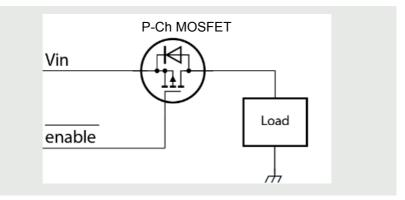
Figure 1 | P-channel MOSFET load switch
