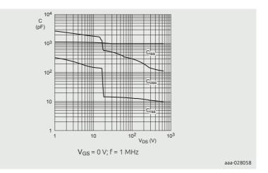
Figure 13 | Input, output and reverse transfer capacitance as a funtion of drain-source voltage; typical values
