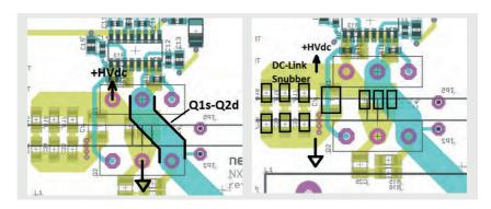
Figure 9 | PCB layout - Detail of power connections Figure 10 | PCB layout - Detail of bypassing: SMD capacitors on PCB backside
