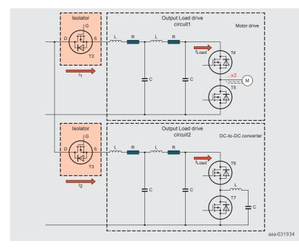
Figure 12 | MOSFETs used as isolators T2 and T3
