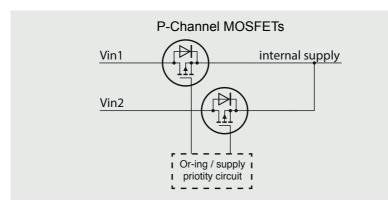
Figure 10 | Power supply OR-ing with P-Channel MOSFETs
