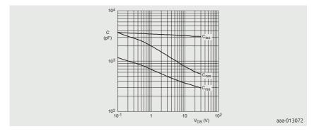
Figure 28 | Input, output and reverse transfer capacitances as a function of drain-source voltage: typical values,  $V_{DS} = 0$  V
