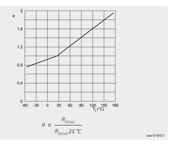
Figure 9 | Normalized drain-source on-state resistance factor as a function of junction temperature
