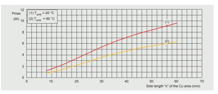
Figure 53 | Maximum permissible power dissipation as a function of copper side length "x" for LFPAK56
