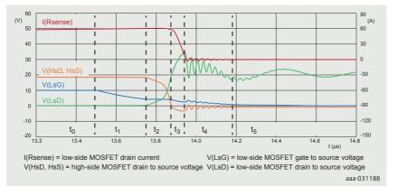
Figure 6 | MOSFET turn-off waveforms, showing reference time periods
