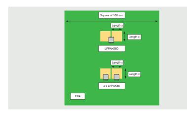
Figure 38 | Copper area configuration: 1 x LFPAK56D, 2 x LFPAK56, single top copper layer
