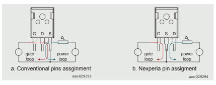
Figure 5 | Illustration of the de-coupling achieved with a centered-source pin assignment
