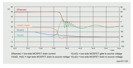
Figure 5 | Turn-on waveform
