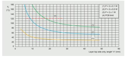
Figure 15 | Junction temperature as a function of copper side length x for LFPAK56D
