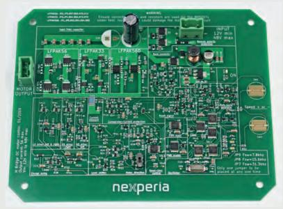
note: gate resistors R57,R58, R78, R79 and jumpers JP2, JP5 are fitted, selecting the MOSFETs in LFPAK56 package
