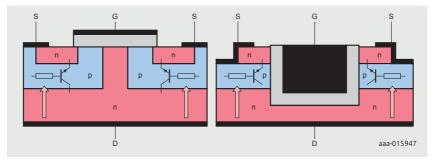
Figure 8 | Simplified planar and trench technology
