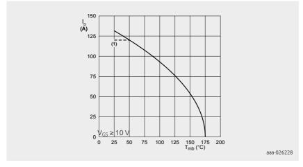
(1) 120 A continuous current has been successfully demonstrated during application tests. Practically the current will be limited by PCB, thermal design and operating temperature.
