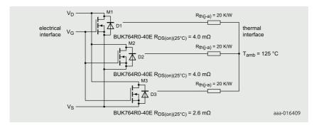
Figure 1 | Electrical and thermal schematic diagram of the three paralleled BUK764R0-40E MOSFETs
