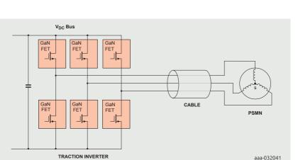
Figure 7 | Traction inverter
