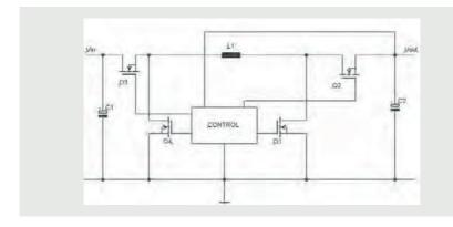
Figure 15 | Up-down converter
