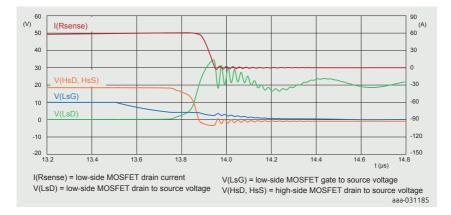
Figure 27 | SPICE turn-off waveform
