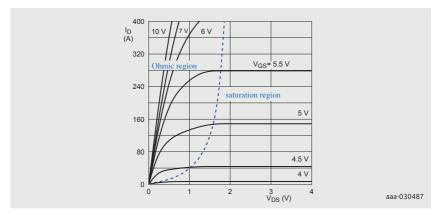
Figure 8 | Example of MOSFET output characteristics
