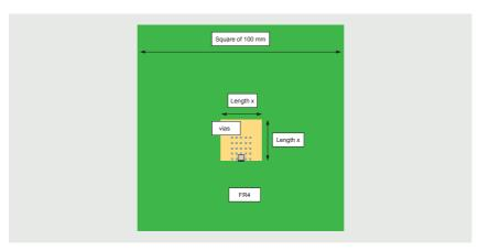
Figure 29 | Copper area configuration: LFPAK33, 4 layers with vias
