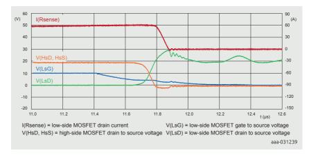
Figure 28 | Measurement turn-off waveform
