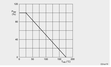
Figure 2 | Normalized total power dissipation as a function of mounting base temperature
