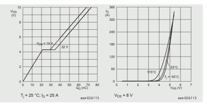
Figure 30 | Gate-source voltage as a function of gate charge; typical values
