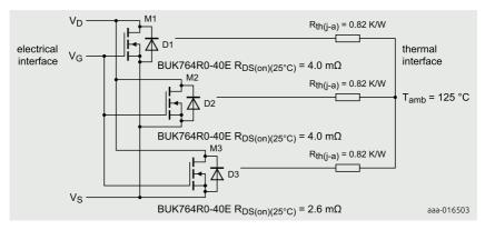
**Figure 2** | Electrical and thermal schematic diagram of the three paralleled BUK764R0-40E MOSFETs with ideal thermal conditions
