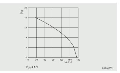
Figure 33 | Continuous drain current as a function of mounting base temperature
