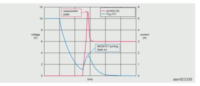
Figure 13 | Blue  $\mathsf{V}_{GS}$  trace shows gate bounce and the red current waveform spiking when gate bounce occurs
