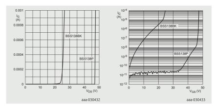
Figure 4 | Gate-source leakage current of ESD protected BSS138BK and non protected BSS138P
