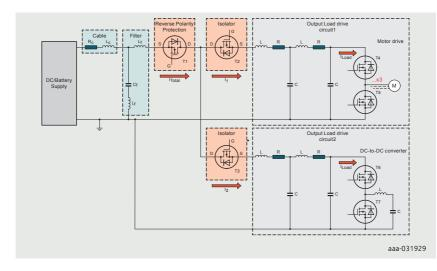
Figure 8 | Simplified motor drive and DC-to-DC converter application diagram
