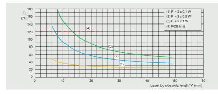
Figure 25 | Junction temperature as a function of copper side length x for LFPAK56D
