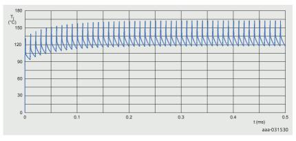
Figure 14 | Inferred junction temperature  $(T_{j})$  rise provided by Figure 12
