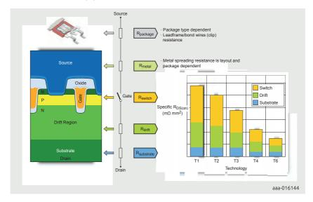
Figure 18 | Resistance in power MOSFETs
