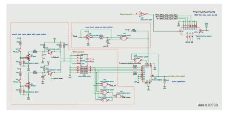
"duty\_cycle\_output" is the general output of the Clock circuit.
