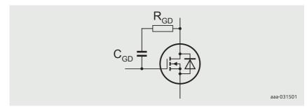
Figure 22 | Adding  $C_{GD}$  and  $R_{GD}$
