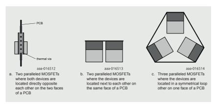
Figure 4 | Good layout arrangements for two paralleled MOSFETs and three paralleled MOSFETs
