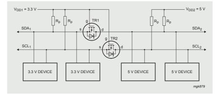
Figure 1 | Bidirectional level shifter circuit connecting two different voltage sections in an I<sup>2</sup>C-bus system
