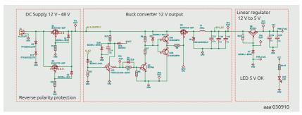
Figure 28 | Power supply schematic
