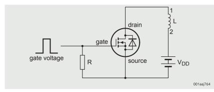
Figure 1 | Unclamped inductive load test circuit for MOSFET ruggedness evaluation
