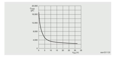
Figure 13 |  $C_{\text{OSS}}$  as a function of  $V_{\text{DS}}$
