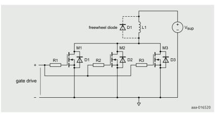
Figure 9 | Low side MOSFET group driving a high side inductive load
