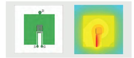
Figure 11 | Test PCB layout 4 and surface temperature profile
