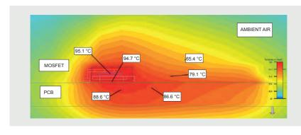
Figure 43 | Thermal result, LFPAK33, 0.5 W, 20 °C ambient
