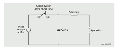
Figure 9 | Oscillation at MOSFET turn-off
