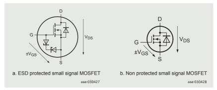
Figure 1 | Illustrated pin configuration for device leakage
