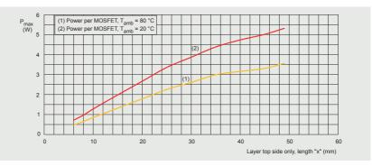
Figure 26 | Maximum permissible power dissipation as a function of copper side length x for LFPAK56D
