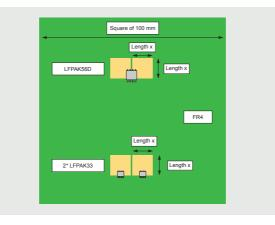
Figure 40 | Copper area configuration: 1 x LFPAK56D, 2 x LFPAK33, single top copper layer
