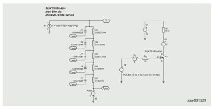
Figure 13 | SPICE circuit illustrating how to integrate an electrical circuit with a thermal model
