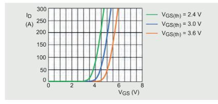
Figure 32 | Transfer characteristic at 25 °C
