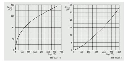
Figure 15 | Typical Q<sub>OSS</sub>
