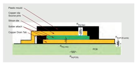
Figure 3 | Thermal resistances inside and outside the MOSFET
