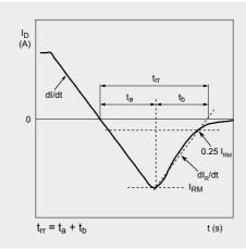
Figure 14 | Reverse recovery waveform definitions
