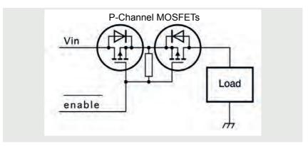
Figure 8 | Reverse current protected common source load-switch
