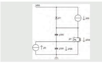
Figure 18 | Diagram for switching behavior tests for MOSFET
