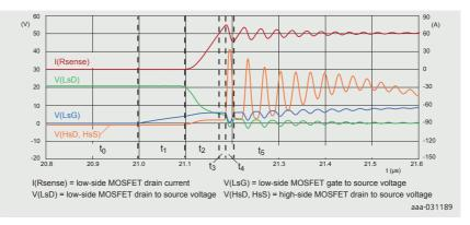
Figure 10 | MOSFET turn-on waveforms, showing reference time periods
