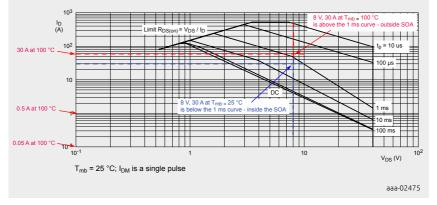
The  $I_D$  derating of the SOA curve at 100 °C is shown in Figure 18.
