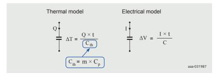
Figure 8 | Thermal and electrical capacitance models
