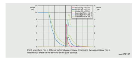
Figure 17 | Effect of  $R_G$  on  $V_{GS}$ , and shoot-through current
