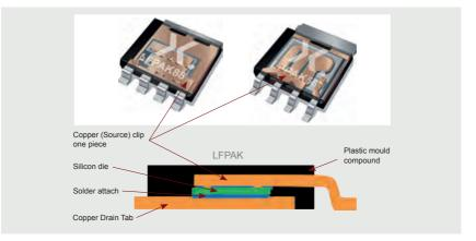
Figure 2 | LFPAK internal structure
