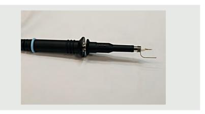
Figure 4 | Oscilloscope probe with ground spring attached
