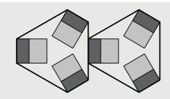
This layout suits standard packaged MOSFETs (e.g. D<sup>2</sup>PAK, LFPAK and TO-220). The dark shaded area corresponds to the drain tab of the device.
