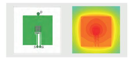
Figure 10 | Test PCB layout 3 and surface temperature profile
