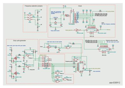
Figure 8 | Clock, duty cycle and frequency selection
