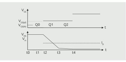
Figure 19 | Turn-on process for MOSFET,  $V_{GS}, V_{DS}$  and  $I_D$  curves
