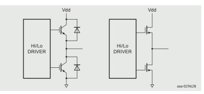
Figure 1 | Comparison of a traditional high-voltage half bridge to a GaN FET half bridge.
