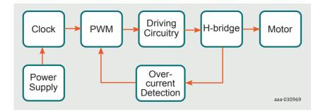
Figure 2 | H-bridge motor controller block diagram
