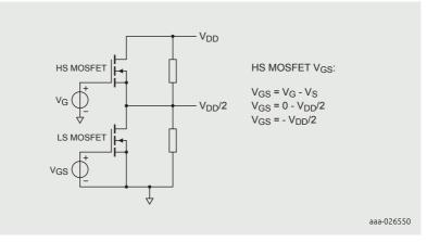
Figure 8 | Half bridge MOSFET configuration showing leakage paths and potential issues if driving High Side MOSFET with respect to ground
