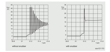
Figure 15 | Effect of adding a snubber
