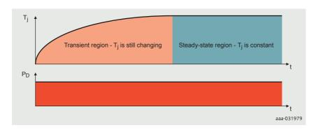
Figure 9 | Transient and steady state thermal behavior
