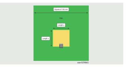
Figure 44 | Copper area configuration: LFPAK56, single top copper layer, the configuration is the same for LFPAK88
