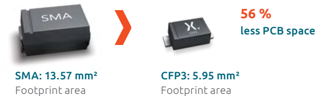
Figure 7: Nexperia Trench Schottky diode in CFP packaging requires only half the PCB space of alternative solutions
